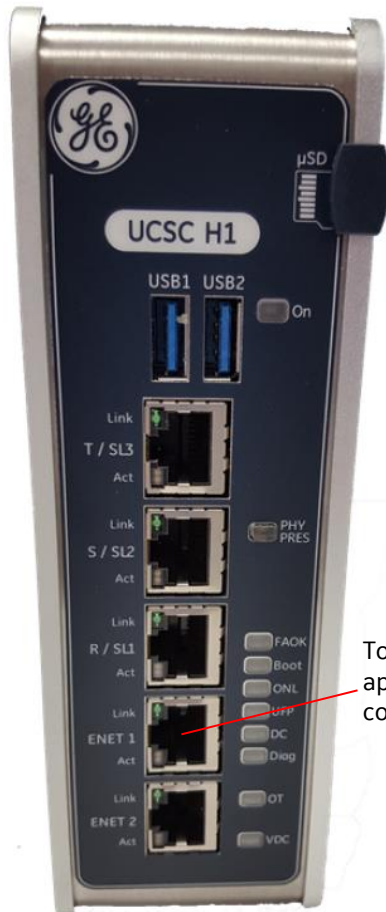
UCSC Controller E1 Connection Simplex configuration
